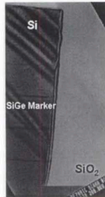
Fig. 3. Cross-sectional TEM images showing the film and mask interface. The undoped film is grown in the window along \langle 100 \rangle .
