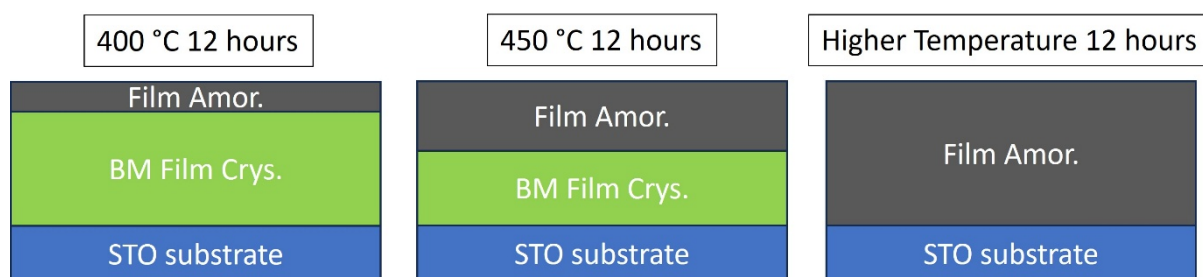
Figure S3.3. Schematic illustration showing the increased amorphous layer resulting from higher annealing temperatures.
